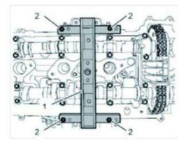
Staking tool screws for cylinder bank "1-3"
