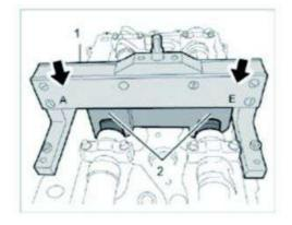
Fitting position of staking tool for cylinder bank "1-3"
