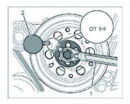
TDC marking on cylinder 1/4 at vibration damper Check position of the outlet sprocket "1".
