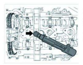
Tightening adjusting screw on staking tool Turn the crankshaft clockwise (running direction of engine) to the TDC marking at the vibration damper.
