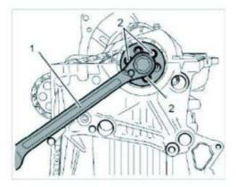
Screw in three fastening screws -2- for the vibration damper at the crankshaft flange.
